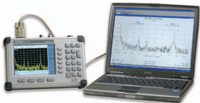
Connect Site Master to a PC via a serial cable to transfer data or further analyze results
